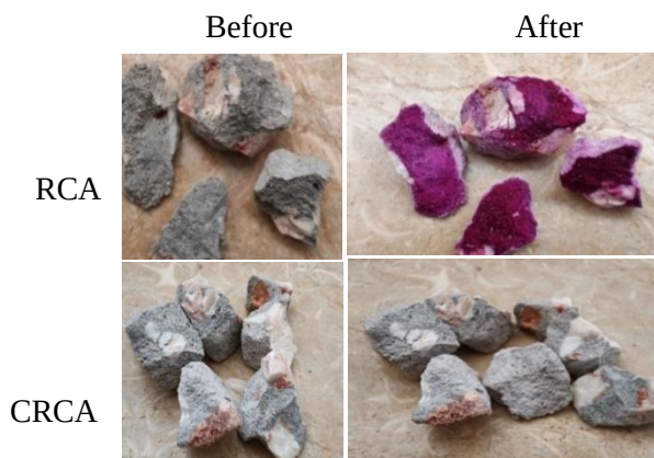
Figure 4. Aggregates before and after spraying the phenolphthalein.
